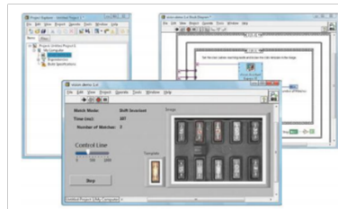
Figure 2. LabVIEW Front Panel, Block Diagram, and Project Explorer in a Vision Development Module Application
