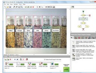
Figure 1. Vision Builder AI Configuration Interface
